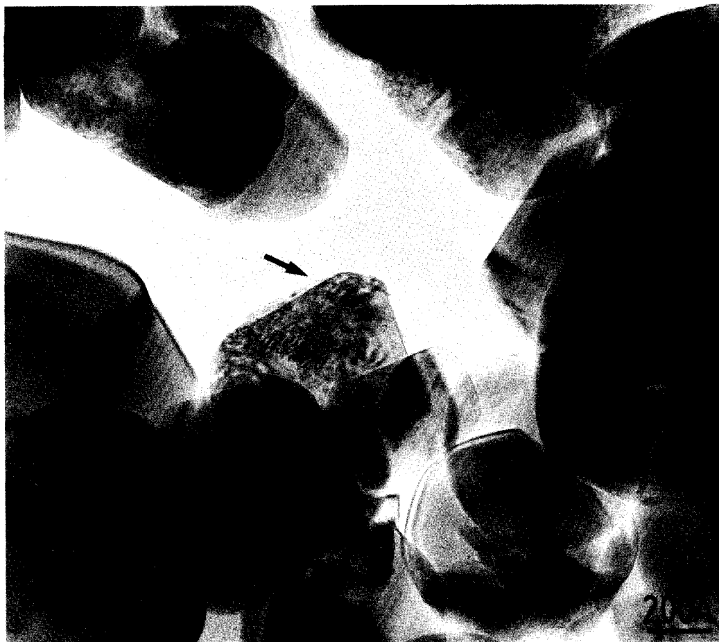
FIG. 6. Typical region of tin-antimony oxide D showing general particle morphology as well as regions of considerable disorder (arrowed).
